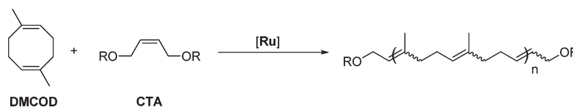
Scheme 1. Synthesis of Telechelic Polyisoprene via ROMP of DMCOD with a Generic CTA
